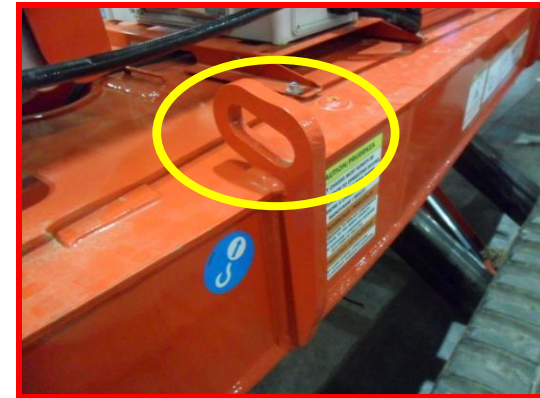
Picture 41: couplings on the frame.
