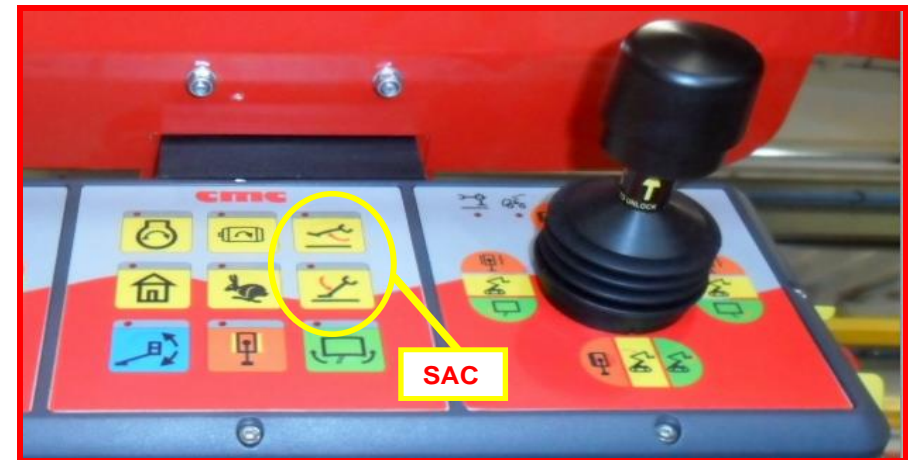
Picture 49: stabilization/destabilization lever on basket station control.
