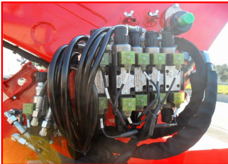
Picture 40: distributor in the emergency workbench.
