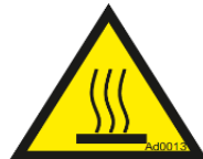
Picture 106: warning of burn risk.
