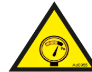
Picture 110: high pressure hazard.
