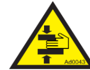
Picture 109: crushing and cutting hazard.
