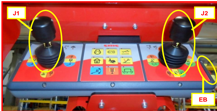
Picture 9: platform control (exercise) station.
